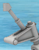
Q48372 Reggiane Re 2000 Tailwheel with Strengthened Leg
