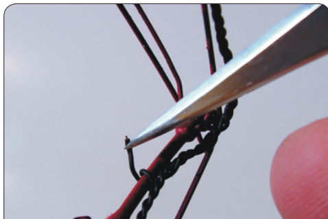
Haltedraht am unteren Pantographen-Holm verdrehen. Twist the lower holding wire around the pantograph.
