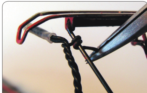
Haltdraht am oberen Pantographen-Holm verdrehen. Twist the upper holding wire around the pantograph.
